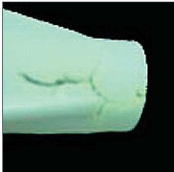
Figure 6. Cracked nozzle from corona.
