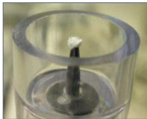
Figure 1. A white "fuzzball" appears on emitter tips as a result of precipitated materials
