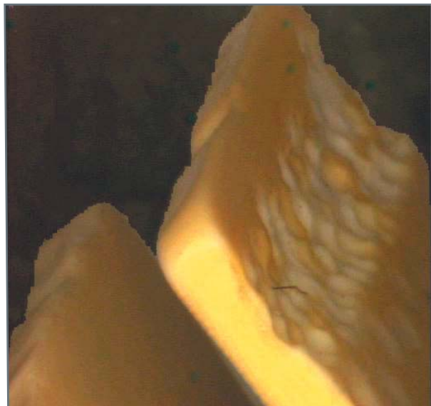
Figure 5. Pitting in emitter nozzle.
