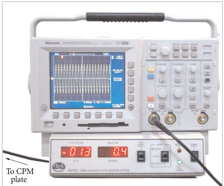
Figure 2. Using a charge plate monitor along with a DSO.
